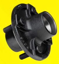
48-979501 Hub & Drum-6000LB CAPACITY 6 X 5.5, 1/2"-20 For 12" Brakes
