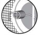
Hook should engage three wires
