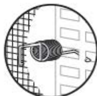
Hook should engage three wires
