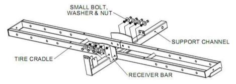
STEP 2. Attach 2 bridge supports and 2 ramp supports as shown using 4 medium bolts and nuts. NOTE: When mounting ramp supports, make sure flat surface is up and the extra 3 inches is on the outside to support the ramp while transporting.
