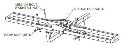
STEP 3. **PLACING THE LARGE BOLTS.** The carrier is designed to load the bike from the left or right side using the ramp. There are 3 sets of center boles and 1 set of upper holes on each cradle. The large safety pins and clevis pins are used in the upper holes. See FIG 5. The 4 large bolts are used in the center hole to support the bike tires. Note: Depending on
