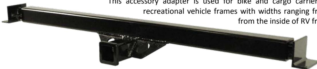
This accessory adapter is used for bike and cargo carriers. Engineered to fit most recreational vehicle frames with widths ranging from 47<sup>3</sup>/<sub>8</sub>" to 77" measured from the inside of RV frame.
